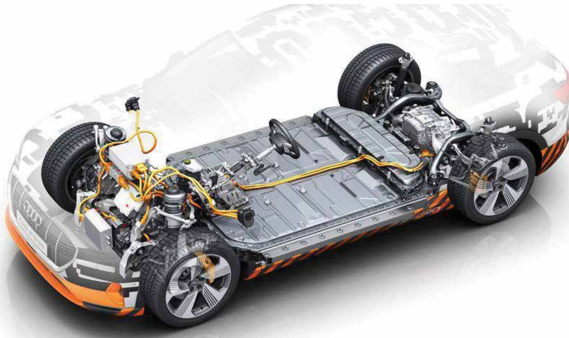
Lithium-ion EV battery, AUDI E-Tron
